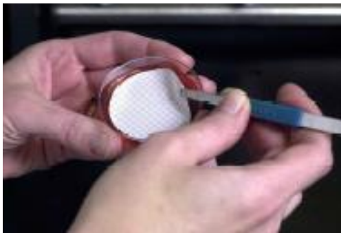
3. Membrane filter is removed from apparatus & placed on agar plate for incubation
